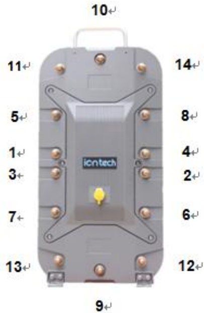
Figure 3-1 Module Tightening Sequence
